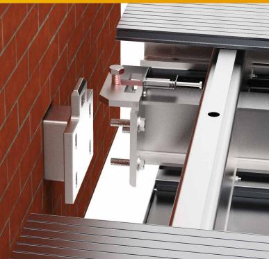
The locking mechanism on the frame is engaged immediately upon landing the balcony onto the bracket. The vertical movement of the red retaining clip will be the sign that the spring bolt has released, locking the balcony to the bracket.
